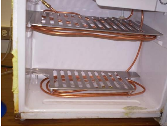
Figure 1 Interior of refrigerator with heat exchanger coils
