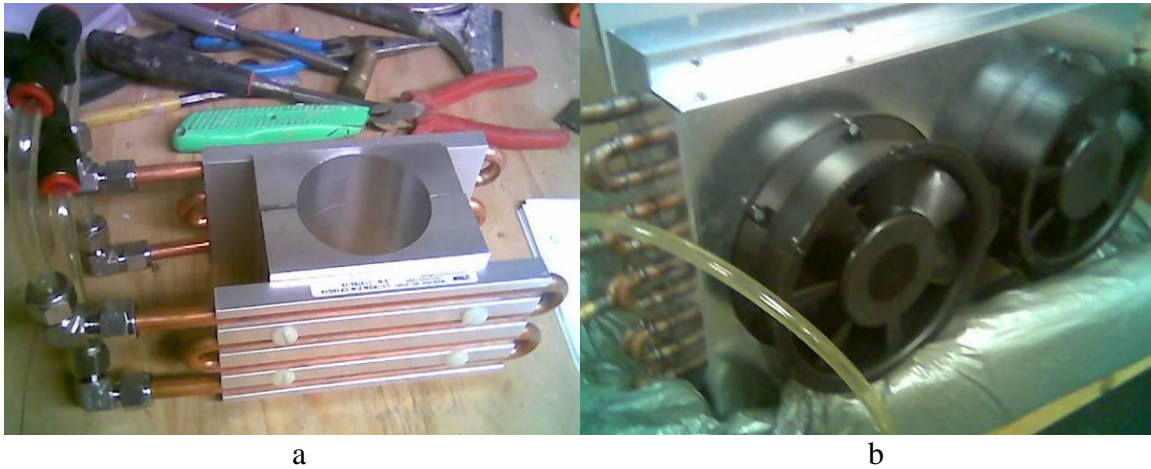
Fig. 2 a) The core with heat exchangers b) The external heat exchanger with fans.
