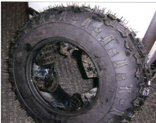
Figure 3a: Internal chambers
