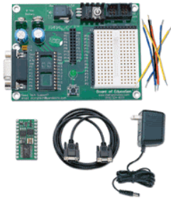
Figure 3: The controller and BASIC stamp.
