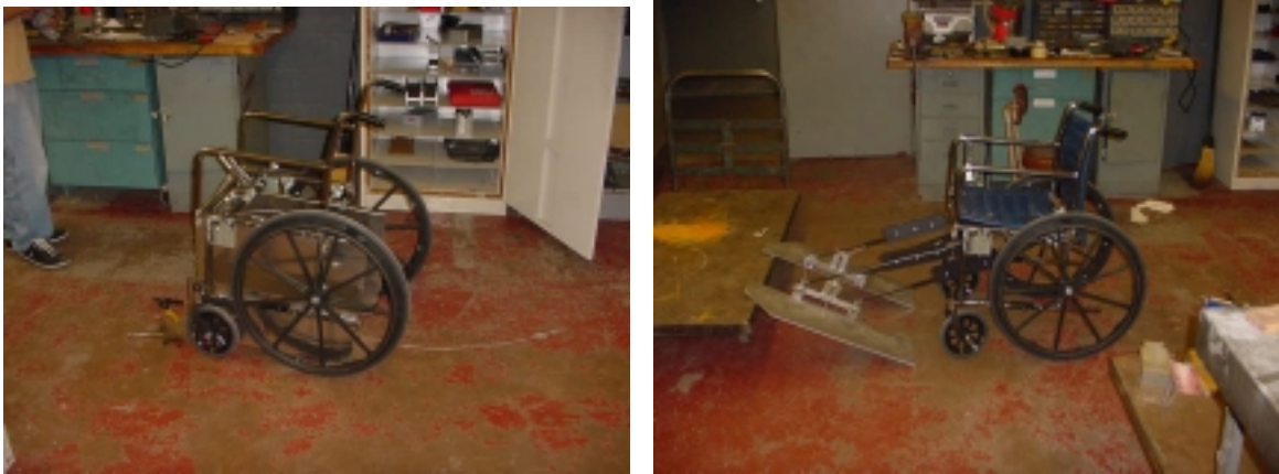
Figure 1: The ramp in home and projected positions.
