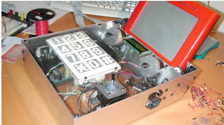
Figure 8: A microprocessor controlled Etch-Sketch for the bi-manually impaired.
