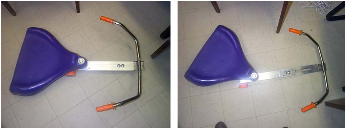
Figure 17: The adjustable Roller Racer in original and extended configurations.
