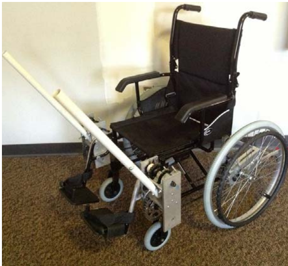
Figure 7. Prototype of One-Step-Climbing Wheelchair
