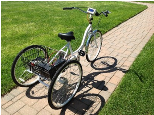
Figure 1. Prototype of Power Assisted Knee Rehabilitation Tricycle
