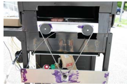
Figure 12. Chain Drive for Flipping Mechanism
