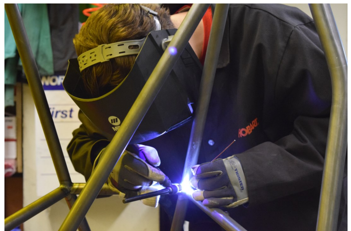
A new tubular frame chassis is created every year. Students notch and weld most of the tubes themselves in our machine shop.
