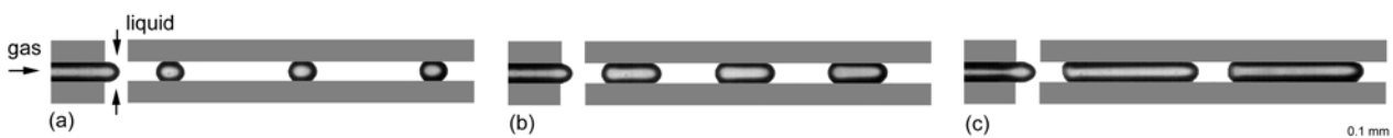
Fig. 3. On-chip mixing section. (a) \alpha_G \approx 0.22 , (b) \alpha_G \approx 0.53 , (c) \alpha_G \approx 0.82 .
