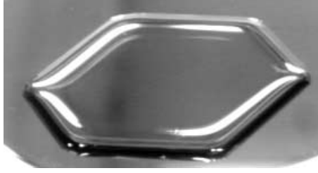
Fig. 5 – Large sessile drop on a hexagonal array of small non-wetting defects ( d = 0.4 mm, f = 0.08 , distance between defects = 0.707 mm), the width of the drop is 6 cm. The defect pattern and contact line motion for this drop are shown in fig. 8.
